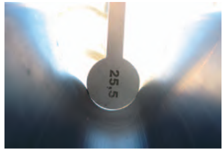
Worn-out sheave: simulated rope diameter -> too small
