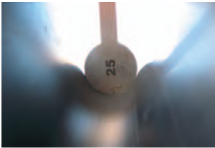
Act. groove diameter 25.0mm
