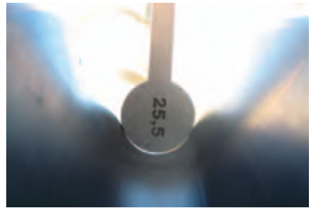
Worn-out sheave: simulated rope diameter -> too small
